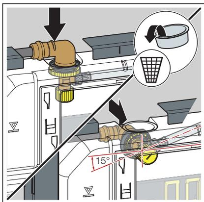
**INFO!** For the concealed cistern 3H, the corner valve can be attached from the top or rear.
