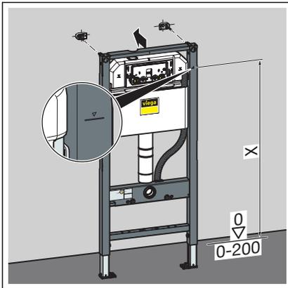
➤ Adjust the construction height of the element in accordance with the on-site marking of the upper edge of the finished floor.
