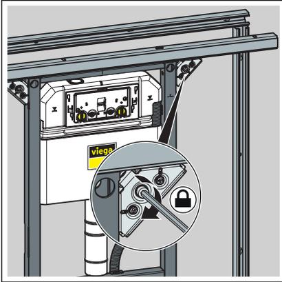
■ Fix the element with the Prevista Dry Plus rail connectors.
