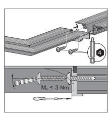
The connection piece 90° is properly mounted when the seal is pushed together gently.
