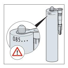
Fig. 5: Filling date of the mounting adhesive
