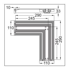
Fig. 6: Dimensions of connection piece 90°
