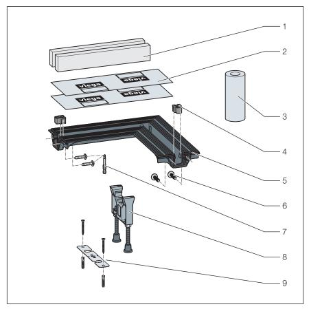
Fig. 3: connection piece 90°, scope of delivery
