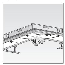
Align shower channel and connection piece 90° both horizontally and perpendicular to one another.
