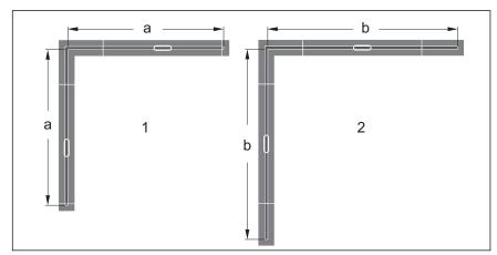
Fig. 1: Installation possibilities with connection pieces 90° for L version
