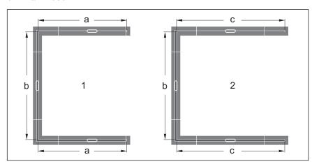
Fig. 2: Installation possibilities with connection pieces 90° for U version
